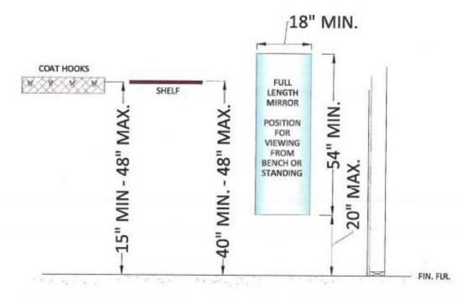
11B-803.6 Mirrors shall be installed with the bottom edge of the reflecting surface 20 inches maximum above the finished floor. Mirrors shall be full length with a minimum 54 inches high by 18 inches minimum width and shall be positioned affording a view to a person sitting on the bench as well as a person in a standing position.
