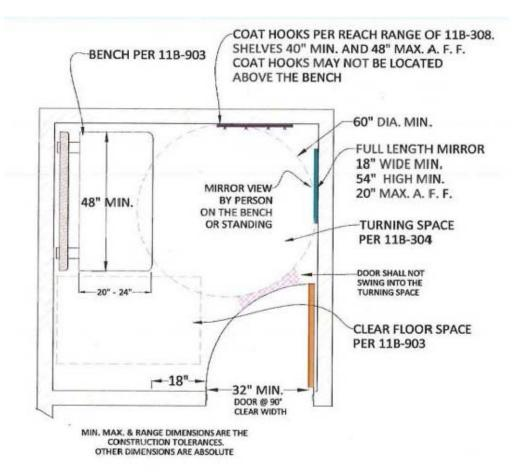
11B-803.5 Coat hooks, when provided shall be within the reach ranges specified in Section 11B-308
