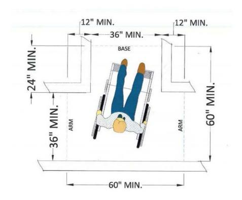
T-shaped shall be within a 60 inch square minimum with arms and base 36" wide minimum. Each arm shall be clear of obstructions 12" minimum in each direction and the base shall be clear of obstructions 24 inches minimum. The space shall be permitted to include knee and toe clearances complying with Section 11B-306 only at the end of either base or one arm.
