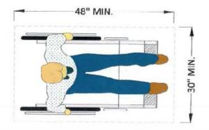
The size of the clear floor space shall be 30 inches minimum by 48 inches minimum
