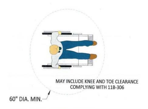
Circular turning space shall be a space of 60 inches diameter minimum and shall be permitted to include knee and toe clearances per Section 11B-306.
