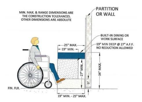
11B-306.2 The space under an element between the finished floor and 9 inches above the finished floor shall be considered toe clearance. Toe clearance shall extend 25 inches maximum under an element. Spaces extending greater than 6" beyond the available knee clearance @ 9" above the finished floor shall not be considered toe clearance.
