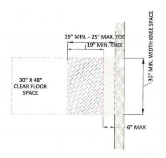
11B-306.3 The space under an element between 9 inches and 27 inches above the finished floor shall be considered knee clearance. Knee clearance shall extend 25 inches maximum under an element at 9 inches above the finished floor.
