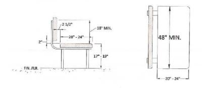
11B-903.2 A clear floor space shall be provided and shall be positioned at the end of the bench seat and parallel to the short axis of the bench.
