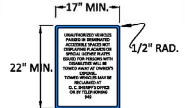
REFLECTORIZED SIGN CONSTRUCTED OF PORCELAIN STEEL WITH BEADED TEXT OR EQUAL
