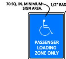
REFLECTORIZED SIGN CONSTRUCTED OF PORCELAIN STEEL WITH BEADED TEXT OR EQUAL
